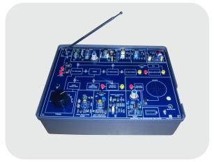
**ACT-09** is a Analog Communication Trainer System to understand DSB/SSB Demodulation Techniques. Various Test points/ functional block diagrams are provided on-board for Teaching/Training.
