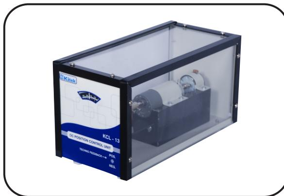
DC position control system is very useful in Controls System Laboratory. This system is easily understood and has a second order transfer function in the standard form, for which a well developed theoretical treatment is available.
