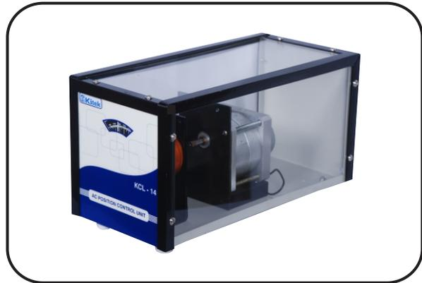
A.C. Position Control System is used in control laboratory experiments. 2-phase ac servomotors have been traditionally used for position/ speed control applications especially in light weight, precision instrumentation areas in airborne systems. The present unit is designed around a 12V ac servomotor and exposes the basic characteristics and dynamics of a position control system.
