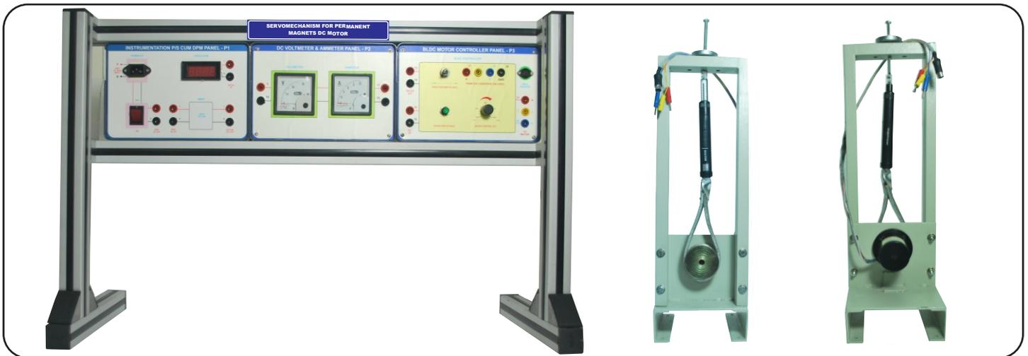
**KMT-02** Brushless DC Motor Trainer is a rugged training system for the Electrical laboratories mounted on Aluminum profile rack with sturdy table top flat panel. Each panel has ABS molded plastic sturdy enclosure with 4mm shrouded connectors showing circuit diagram & its connection tag numbers for easy understanding and connections. The product helps you to get fully acquainted with the basic concepts and functioning of an Brushless DC Motor.
