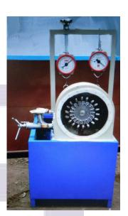
transparent using Perspex to allow observation of turbine during operation. The unit is a compact and designed for quick and easy setting up of experiments. All components and instrumentation are placed in robust and mobile frame.
