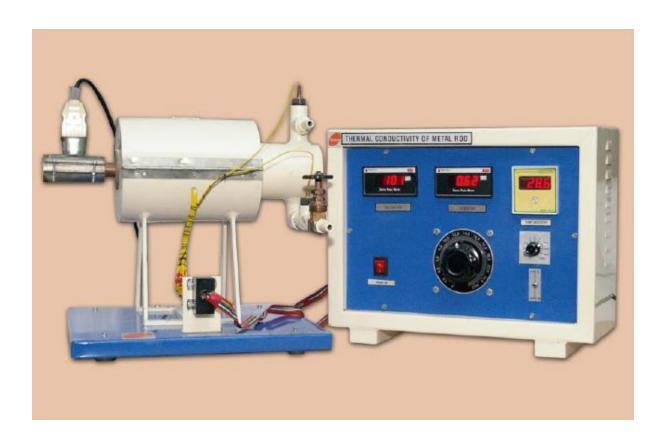
The Thermal Conductivity of Metal Bar Apparatus Model KHT-007 demonstrates the principle that thermal conductivity is a physical property of materials, indicating the ability of a substance to transmit thermal energy through molecular motion. This apparatus provides a clear and practical method for studying heat conduction in solids.
