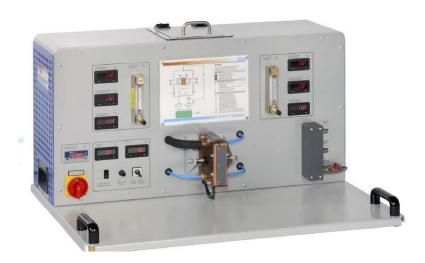
**Cooling Using Peltier Effect Apparatus Model KHT-051** is designed to demonstrate cooling using the Peltier Effect (Thermoelectric Effect). The central component of the system is a Peltier element. When current flows through the element, one side becomes hot while the other side becomes cold. The heating and refrigeration capacity of the Peltier element are dissipated via water flows.
