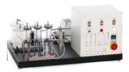
Catalysts enable or accelerate chemical reactions. The **Fixed Bed Catalysis Apparatus Model KHT-165** is designed for the decomposition of dissolved saccharose into glucose and fructose.
