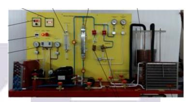
Sight glasses at inlet and outlet of evaporator and condenser allows students to monitor changes in refrigerant state. The system components are panel mounted to provide easy access for testing and troubleshooting.
