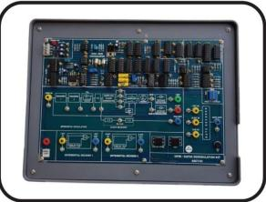
ADCT-XX is an Advance Digital Communication Trainer System that helps one under stand various Digital Modulation and Demodulation Techniques. Various functional block diagrams are provided on-board as an aid for Teaching/Training. These Kits are provided with various Test Points to visualize the signals on Oscilloscopes.
